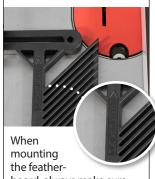
board, always make sure that the "FEED DIRECTION" is pointing toward the cutter. This will make sure the fingers of the featherboard will work properly
