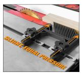
With the expanding miter bars installed onto a feather-board, place the featherboard expanding miter bars into a standard 3/4" x 3/8" miter slot. Place slight, equal pressure on the featherboard toward the stock and fence and secure the knobs. The featherboard should not lift out or slide once it is secure. If it does, you must adjust the notch on the bolts so that they seat inside the slots properly on the expanding miter bar.
