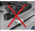
Some table tops may not be large enough to handle this featherboard system. The featherboard must always be sitting flat against the table with no overhang of the miter bars. If there is overhang, DO NOT USE the featherboard on that table top.
